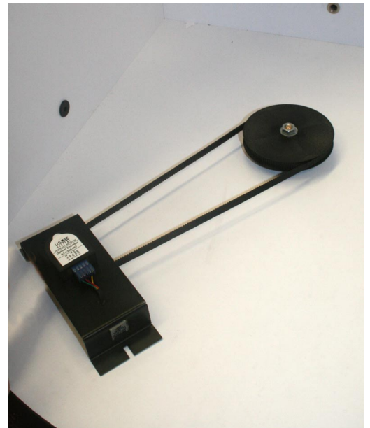
Fig. 2 Timing belt installation
